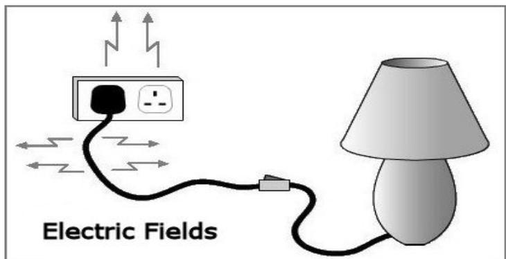
The electric fields are present all the time electricity is present in the wire, even if the electricity is not actually being used.
