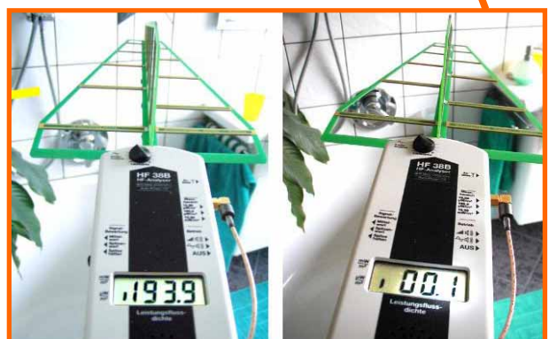
6) Point of measurement marked; power flux density in \mu\text{W}/\text{m}^2 ; before shielding: after shielding:
