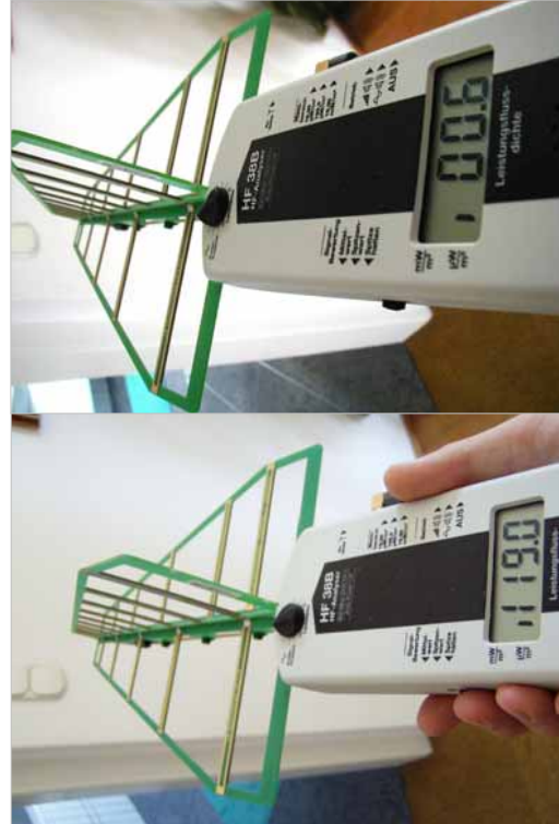
Hallway, first floor; before shielding = 119.0 \mu\text{W}/\text{m}^2 ; after shielding = 0.6 \mu\text{W}/\text{m}^2
